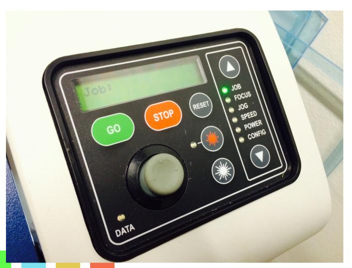
Make sure that the Job menu is active On the display screen, the name of the file sent should display right under Job:
