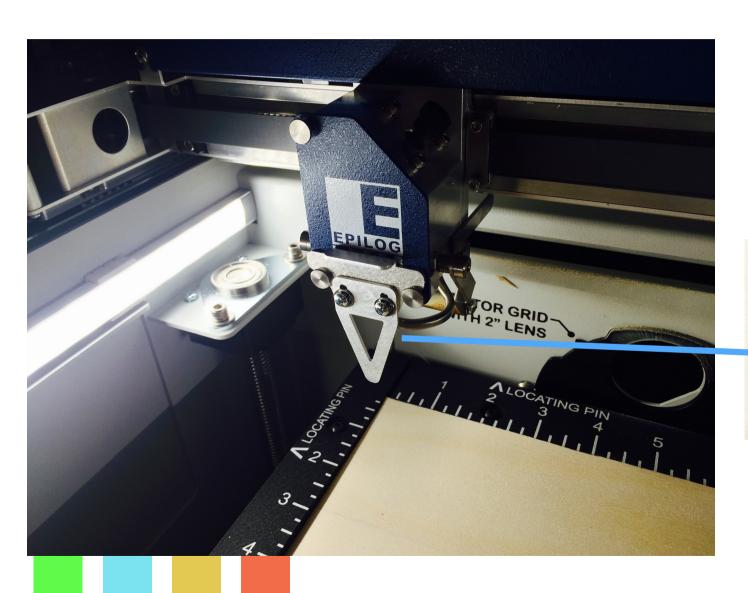
After the height calibration, remove the calibration piece and put it back in the tray
